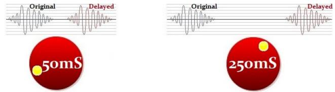
If we add the delayed signal to the original signal, it sounds like an echo. How late the echo sounds will depend on the **Delay Time** you set.
