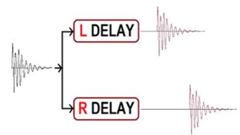
Effect Units are often in **Stereo**. There will be one input and two outputs (usually called L and R out). Stereo offers you two distinct Delay Units, so you can have a different Delay Time and a different amount of Feedback on each channel. This creates a very full sense of space.
