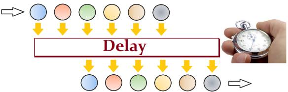
A Delay Unit (originally called a Delay-Line) makes a recording of the soundwave arriving at it's Input connector, then it waits a moment (*Delay Time*), and then plays the sound through to its Output connector.
