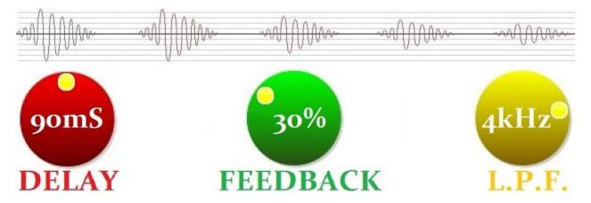
Feeding back a sound often accents the high frequencies, and the result can become quite bright and metallic sounding. Delay Units usually offer some form of high cut filter (Low Pass Filter) to control this. Feedback usually sounds at its best with the high frequencies lowered slightly. Start with a high number (eg. 15kHz) and slowly turn it back down below 10kHz, listening for the point where the bouncing echoes are still audible but are warmer sounding than the original sound is.
