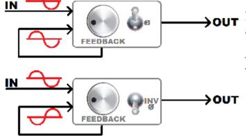
At the moment of feeding back some of the output to the input you may have the chance to invert the signal. **Inverting the Feedback** will cause clashes with the phase (cancellations and boosting) of the arriving signal.
